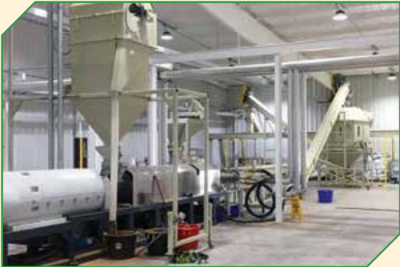
The Diamond Nutrition pellet mill extrudes dried distillers grains (DDG) from the ethanol plant into range cubes and calf pellets.
